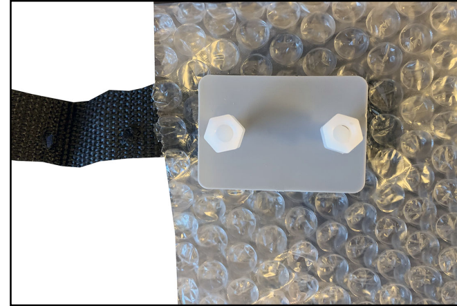
#8 : Place second plate on top and fasten with nylon nuts
