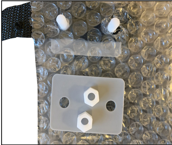
#7 : Insert nylon screws through plate, strap and solar blanket
